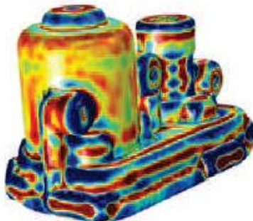
Temperature distribution on cooling surface
