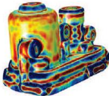
Temperature distribution on cooling surface
